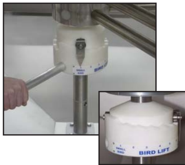
Lower cam adjusts for flock variance
